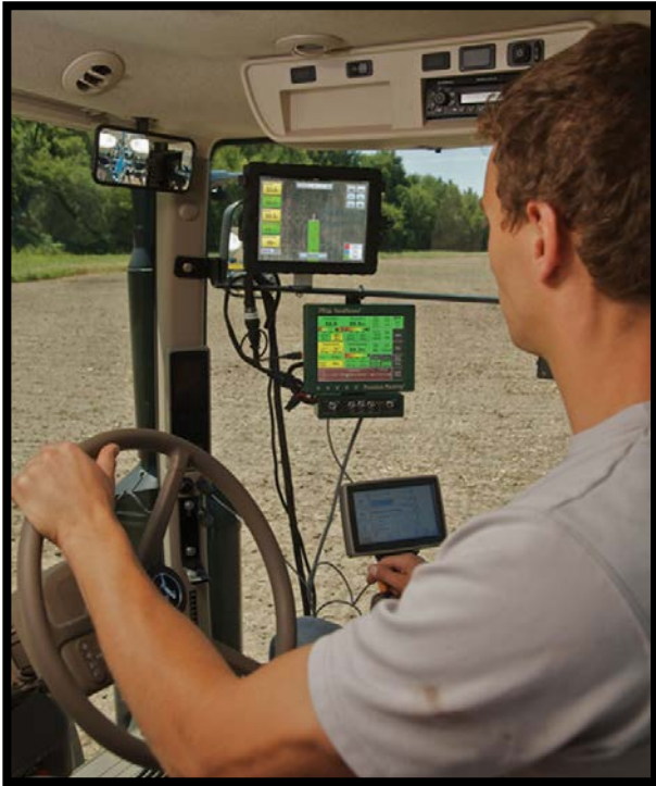
Figure 2 – In-cab precision agriculture system. Photo Credit: modernfarmer.com
