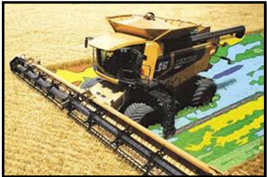
Figure 3 – GPS yield monitor collecting spatially explicit yield data. Photo credit: innovativegis.com
